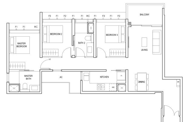
FULL HEIGHT ALUMINIUM FIN LOCATED AT LEVELS: F1 - #03 to #18 F2 - #05, #06, #09, #10, #13, #14, #17 & #18 F3 - #03, #04, #07, #08, #11, #12, #15 & #16
